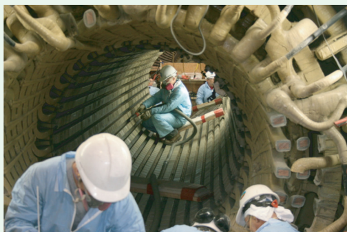
Figure TF26-4: Maintenance technicians working inside one of the generator coils at the Intermountain Power Project, a coal-fired power generation station. (Photo courtesy of Intermountain Power Project.)
