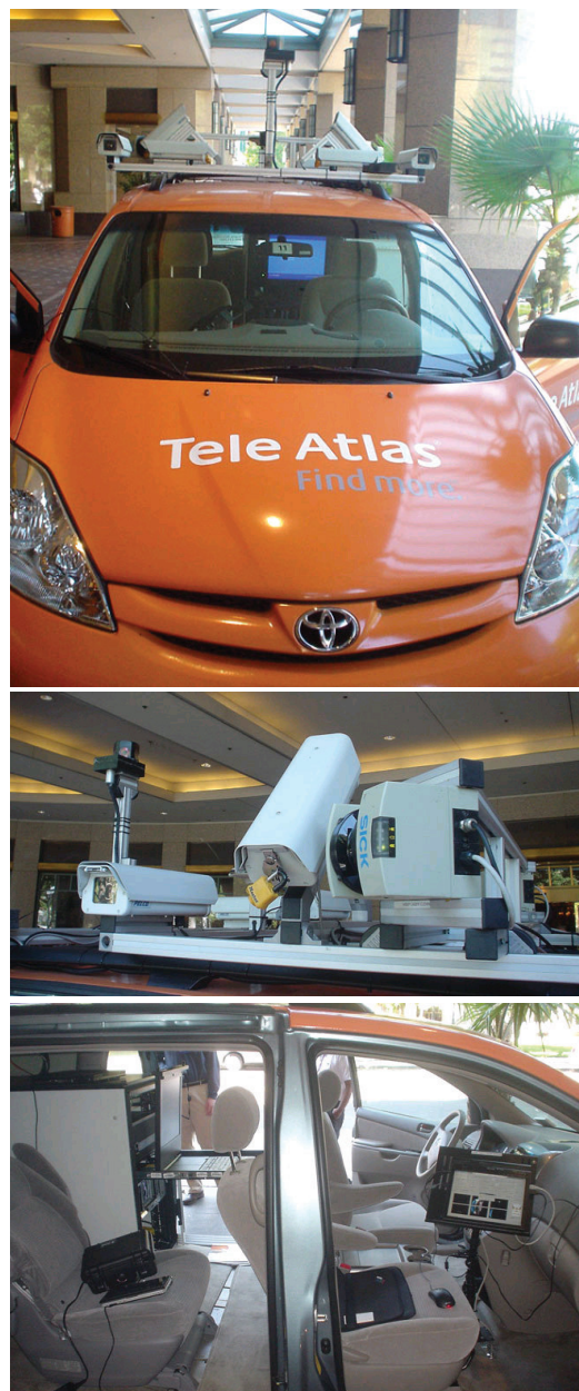
Figure TF29-3: A TeleAtlas van showing the imaging and laser equipment and the computation hardware inside the van.
