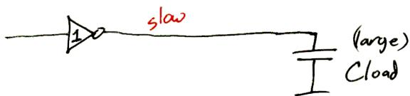
Inverter (base size) is small  $\rightarrow R_{out}$  is large,  $C$  is large, so delay is really long. ( $R_{out} \cdot C_{load}$ )
