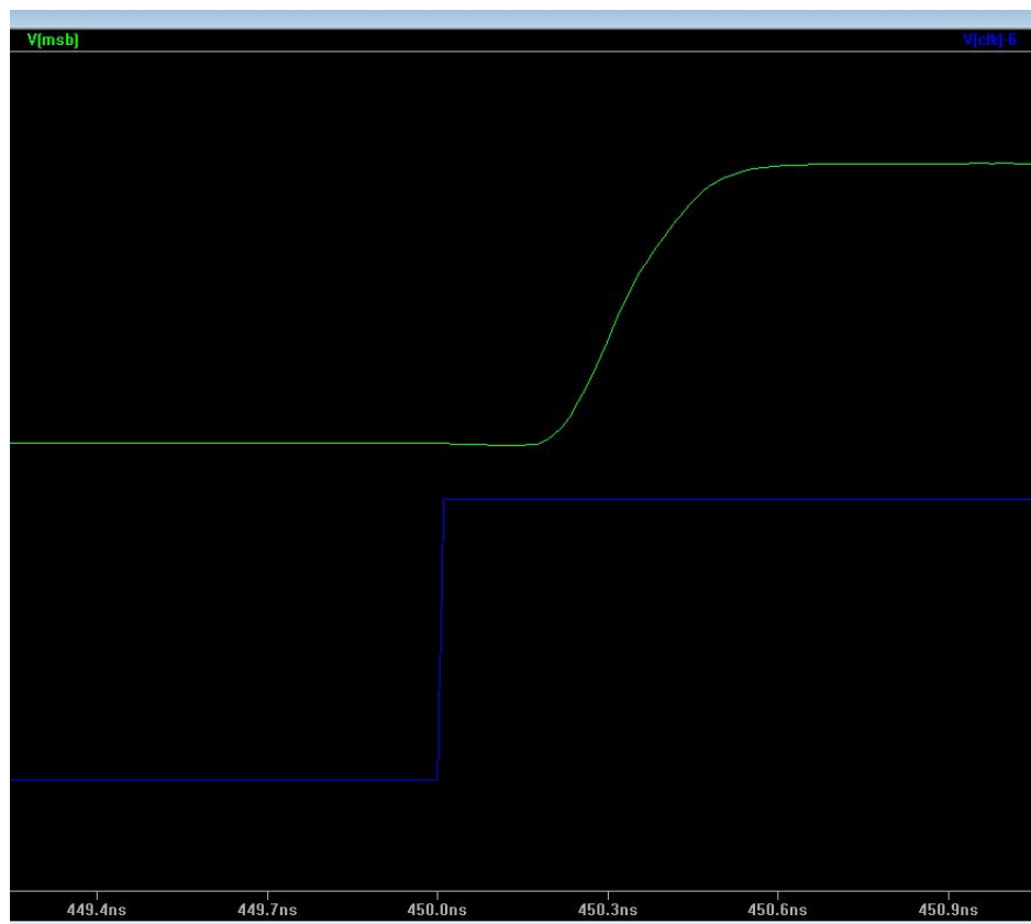
Figure 13: Clock to Q delay for NCO: 0.385 ns - Schematic
