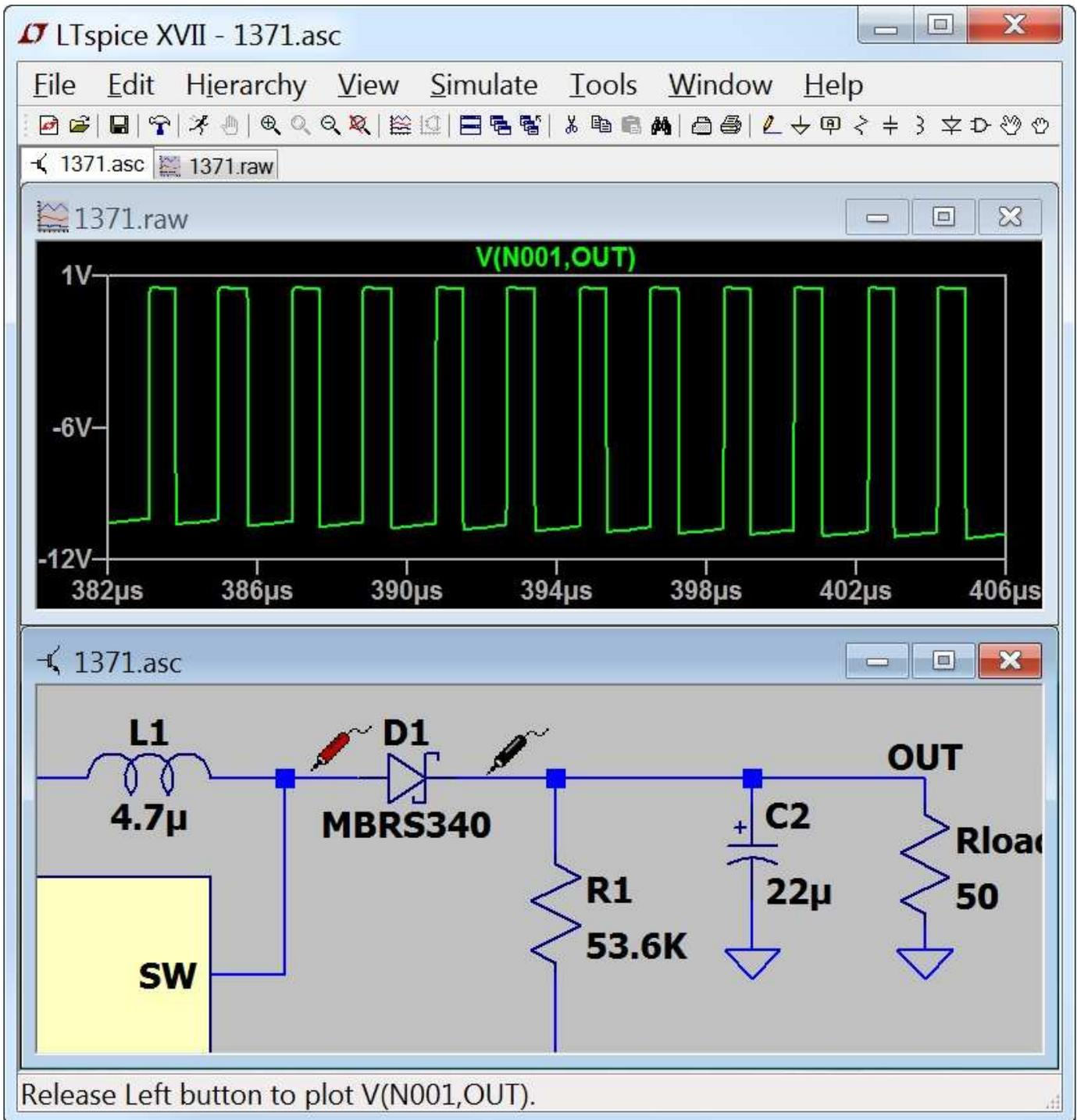
Yet another schematic probing technique is to plot the instantaneous power dissipation of a component. To do this, hold down the Alt key and click on the body of the symbol of the component. The instantaneous power dissipation will be plotted as an expression of voltages and currents. It will be plotted on its own scale with the units of Watts. The mouse cursor turns into an icon that looks like a thermometer when it's pointing at a dissipation that can be plotted. You can find the average
