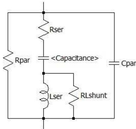
**Capacitor Instance Parameters**
