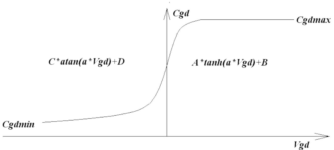
For positive  $V_{gd}$ ,  $C_{gd}$  varies as the hyperbolic tangent of  $V_{gd}$ . For negative  $V_{gd}$ ,  $C_{gd}$  varies as the arc tangent of  $V_{gd}$ . The model parameters  $a$ ,  $C_{gdmin}$ , and  $C_{gdmax}$  parameterize the gate drain capacitance. The source-drain capacitance is supplied by the graded capacitance of a body diode connected across the source drain electrodes, outside of the source and drain resistances.
