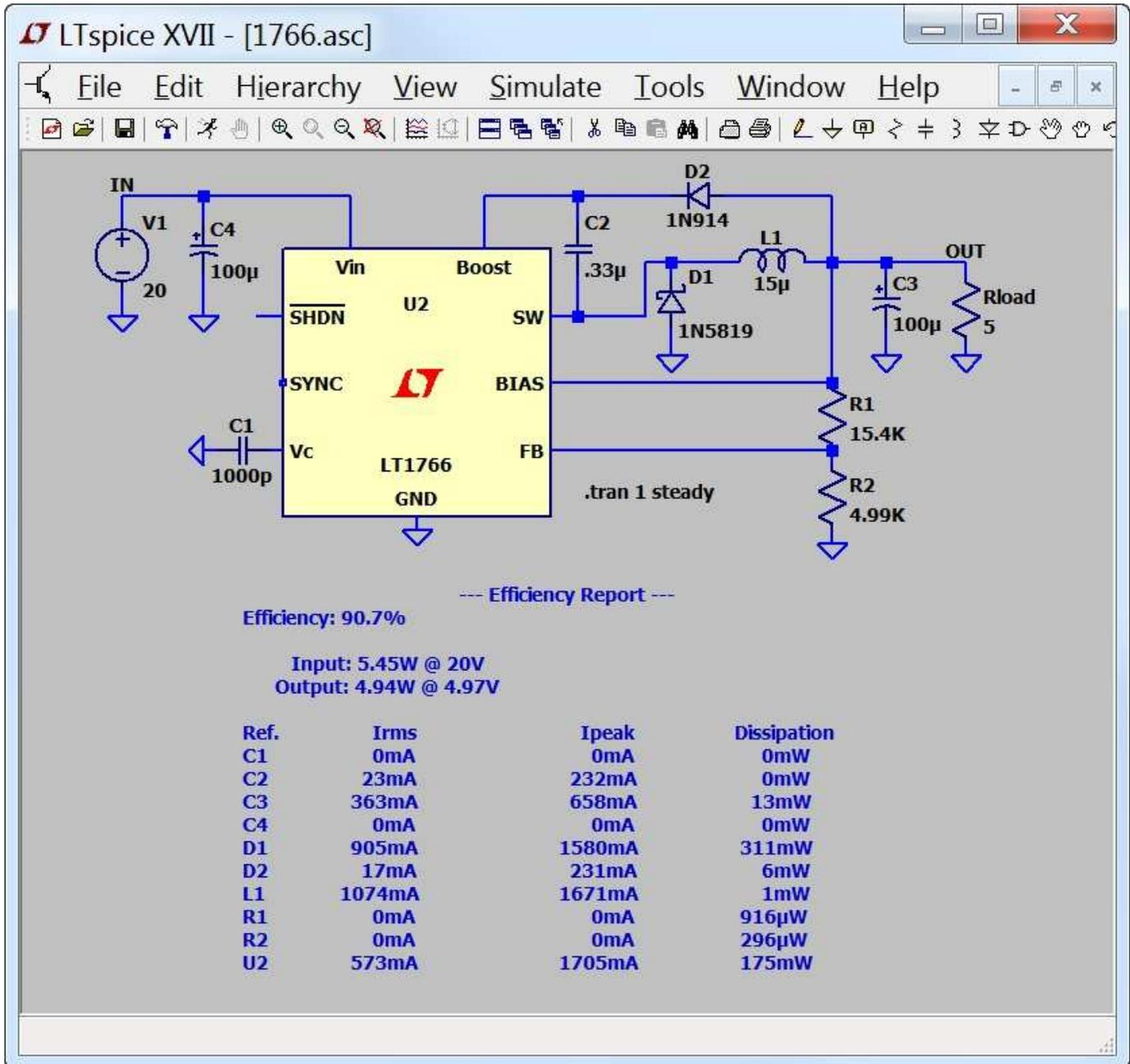
The efficiency of the DC-DC converter is derived in the following manner. In order to identify the input and output, there should be exactly one voltage source and one current source. The voltage source is assumed to be the input while the current source is
