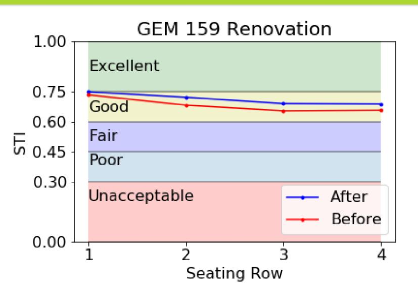
The ranges above are the standard set used for acoustical analysis. Each of the data points is 24 recordings averaged together. You can see how much the data varied below. According to our results GEM 159 has improved slightly and is within the standard good range. However, if either the speaker or the listener's first language is not English, common in collage classrooms, then good just isn't good enough. Why settle for good when you can be excellent?
